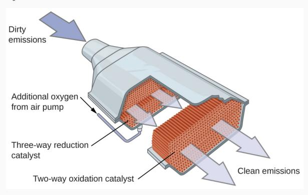
Most modern, three-way catalytic converters possess a surface impregnated with a platinum-rhodium catalyst, which catalyzes the conversion of nitric oxide into dinitrogen and oxygen as well as the conversion of carbon monoxide and hydrocarbons such as octane into carbon dioxide and water vapor:
